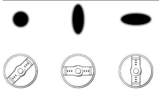
Your spray gun offers you many options. You can adjust (click) the air cap to three positions. One will produce a horizontal pattern for spraying across, another will produce a vertical pattern for spraying up and down, and the third will produce a round pattern to spray small areas such as arms or the face.
